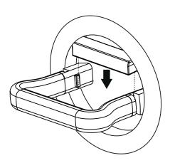
Insert and position the safety connector into the round space.
