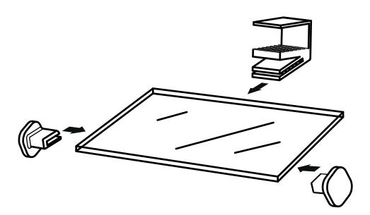
Add double sided mounting tape to the two fasteners that hold the mirror in the inner side panels of the hive.
