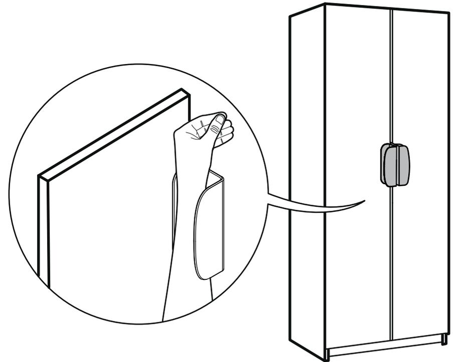
It is recommended to add double sided mounting tape in the inner part of the handle that connect to the closet's door.
